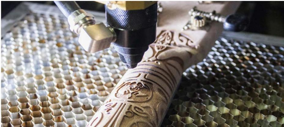
Not all projects are perfect flat pieces of material. Some applications might have uneven surfaces. In this case, one might be confused on how to focus the laser for the best output onto a given item.
