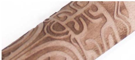
When a design comes out of focus range, the output will become blurred, distorted and/or faded.
