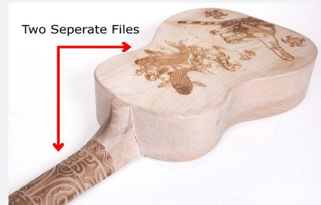
**Breaking Up Uneven Surfaces** Some designs will have to be broken up into separate files. If a given project has two different heights that are outside of 1/8 of an inches of difference, then you will have to break up your design into multiple files and focus and cut each separately.
