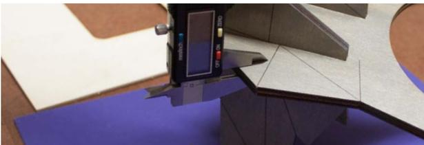
When creating notches, an accurate measurement of the material height is crucial. Because material can vary in thickness, we recommend using calipers to get a precise measurement.
